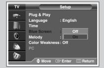
If no signal is being received or the signal is very weak, a blue screen automatically replaces the noisy picture background. If you wish to continue viewing the poor picture, you must set the "Blue Screen" mode to "Off".
